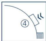
You start a measurement by pressing the start/stop pusher ④ at 2:00 o'clock. The large stopwatch second hand ⑤ is immediately set into motion. After 60 seconds, the hand of the 30-minute counter ⑥ moves to the next index, and the hand of the 12-hour display ⑦ moves a tiny bit farther.
