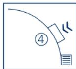
You start a measurement by pressing the start/stop pusher (4) at 2:00 o'clock. The large stopwatch second hand (e) is immediately set into motion. After 60 seconds, the hand of the 30-minute counter (f) moves to the next index.
