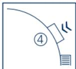
In order to interrupt the measurement, press the start/stop pusher ④. By pressing it again, you continue the measurement.
