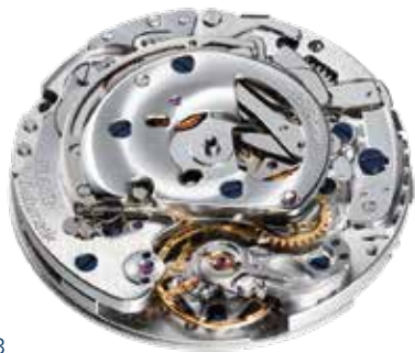
MU 9413 Automatically wound with a woodpecker neck regulation, Glashütte three-quarter plate and Mühle rotor (removed in the image). Ø 30.0 mm; H 7.9 mm. 48-hour power reserve. Functions: hour, minute and small second with stop-second; chronograph with stop-second, 30-minute and 12-hour counters, fast date correction and, where applicable, weekday correction. Characteristic Mühle surface finishes with blued screws, Glashütte solarisation and perlage.
