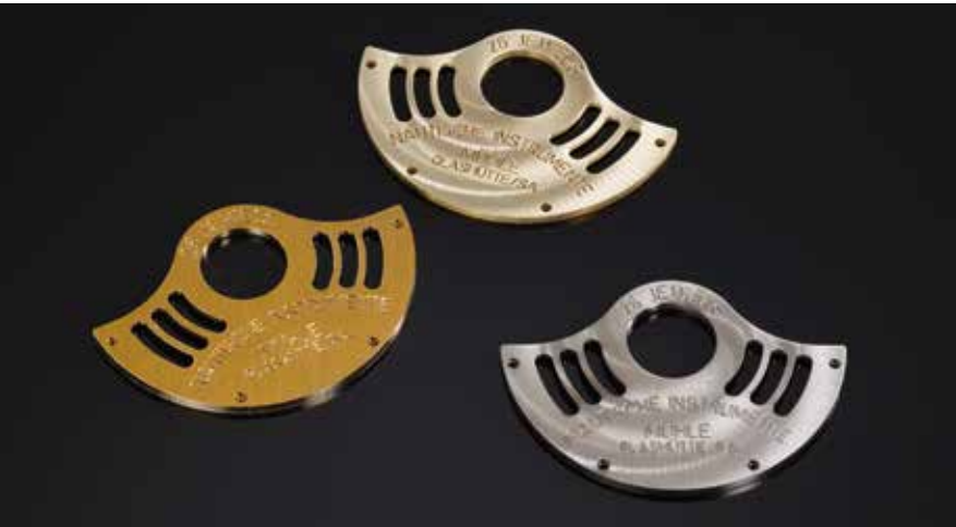
The development of a Mühle rotor (from left to right): a brass blank from parts manufacture, a deburred middle segment with Glashütte solarisation and a finished rhodanised middle segment
